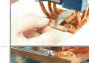
Place SilentTower on the CPU core (Please note the direction of the placement).
